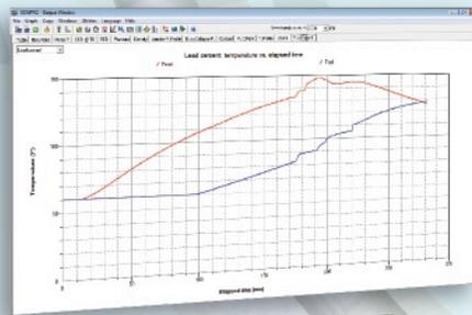
Slurry Temperature vs. Elapsed Time
