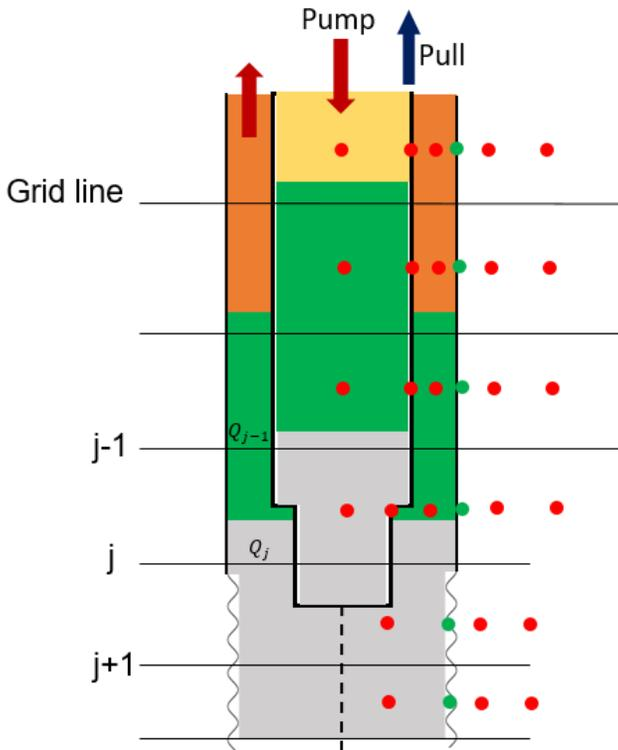
Figure 1: An illustration of wellbore structure with grid lines and calculation points shown for temperature modeling of pulling out of the hole. The red dots indicate the centers of the mesh cells used in the model. The green dots indicate the location of the borehole wall. Q's are flow rates found at the cell faces.
