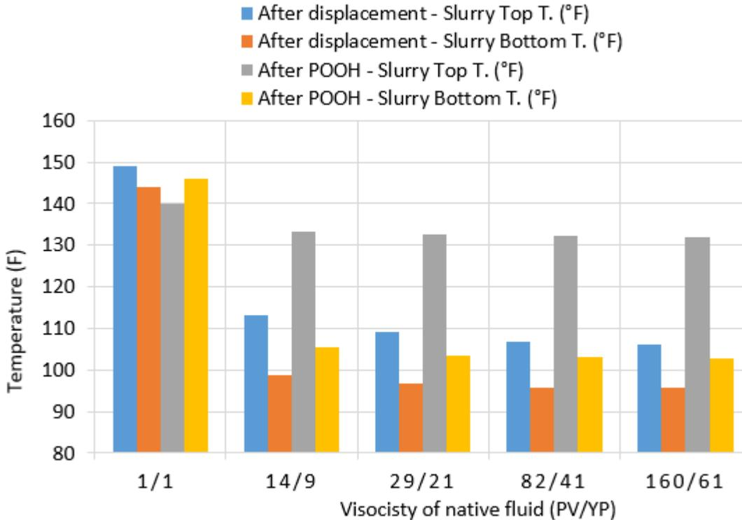
Figure 18: Effect of native fluid viscosity. The units are cP and lbf/100ft<sup>2</sup> for PV and YP, respectively.
