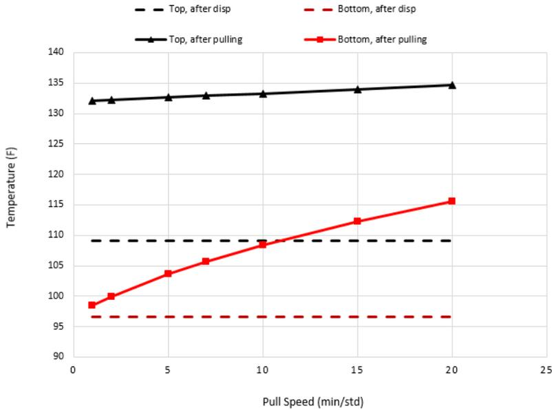
Figure 16: simulated slurry temperature after pulling out of the hole via different pulling speeds.
