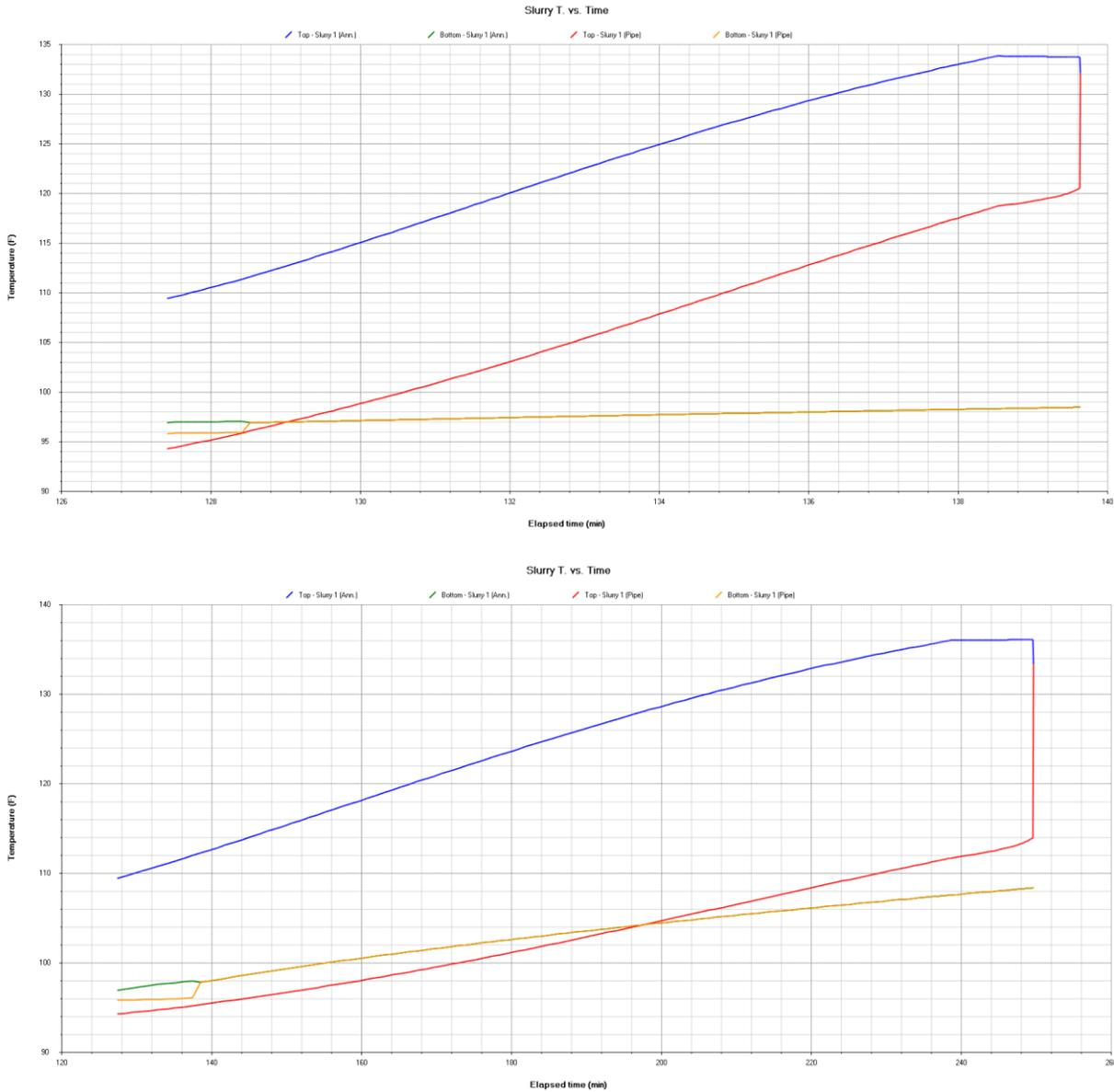
Figure 15: history of slurry temperature while pulling pipe at a speed of (a) 1 min/std; (b) 10 min/std.
