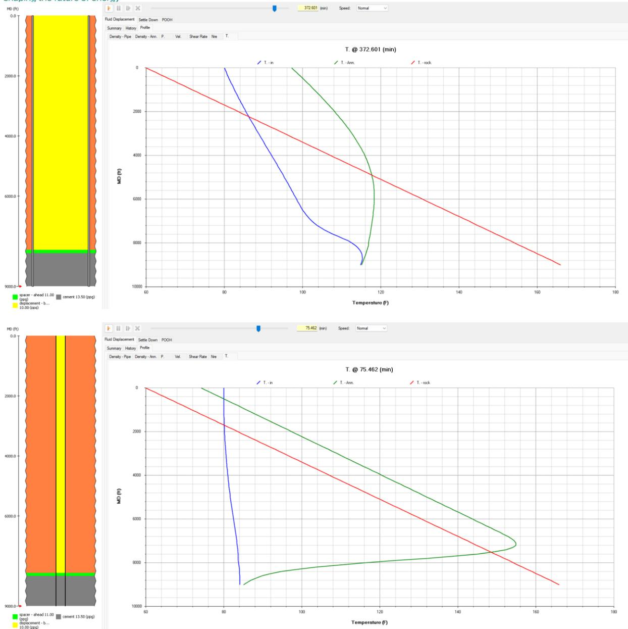
Figure 13: a comparison of temperature profiles after displacement between large and small pipes (top:11.75/11 in; bottom 2/1.782 in)
