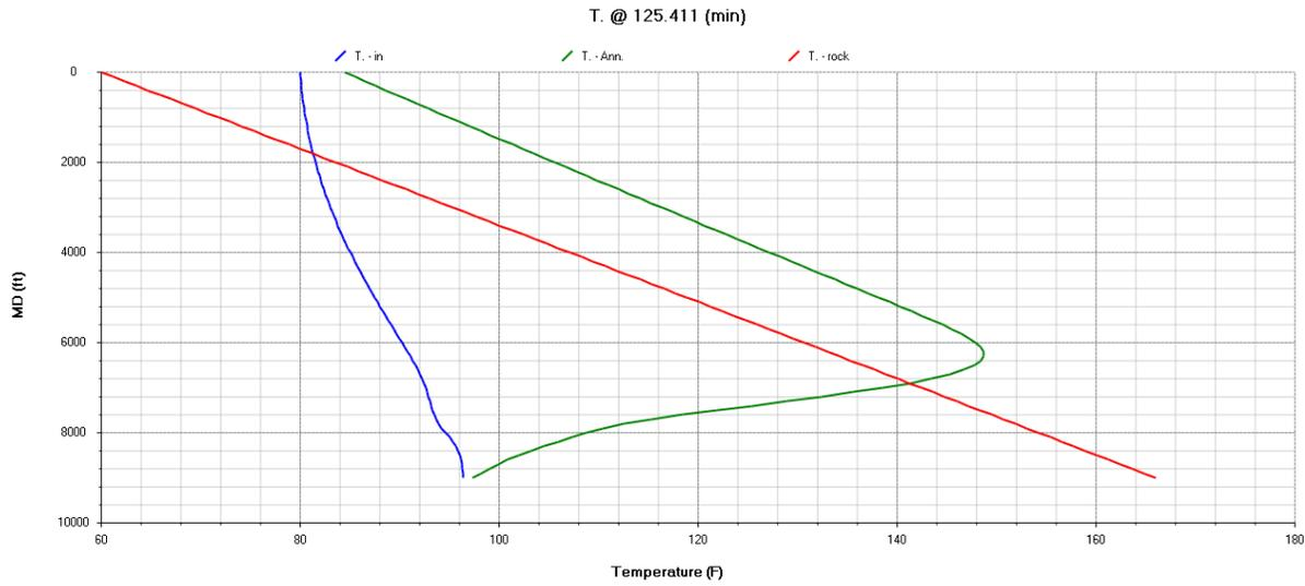
Figure 9: temperature profile after displacement. BHCT is at approximately 97F.
