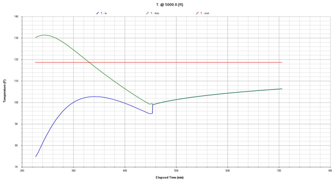
Figure 6: temperature history at 5000'. The T-in and T-ann merges to the same temperature at about 450 minutes, when the pipe end is pulled to the depth of 5000'.
