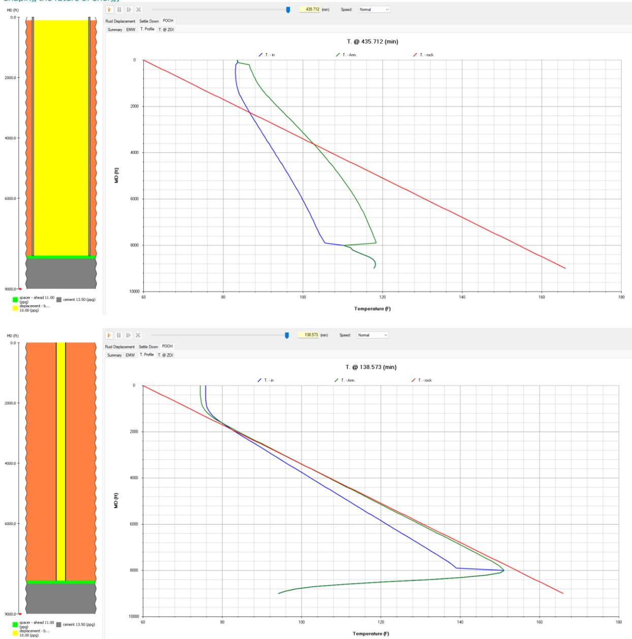
Figure 14: a comparison of temperature profiles after POOH between large and small pipes (top:11.75/11 in; bottom 2/1.782 in)
