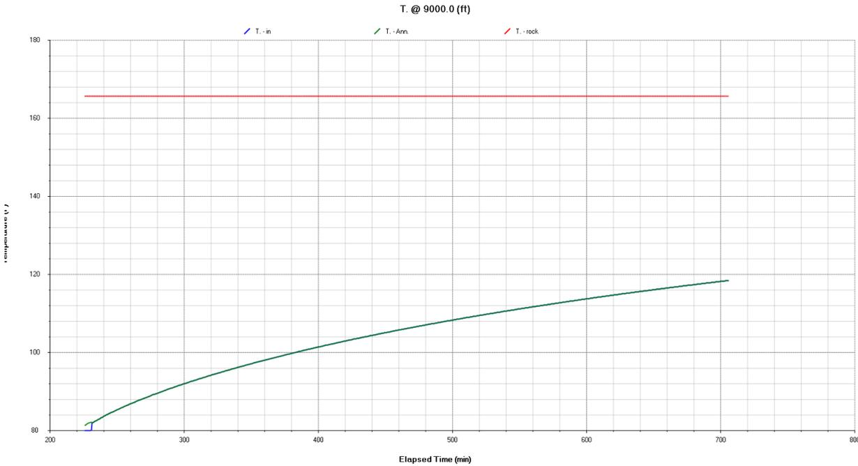
Figure 7: temperature history at the well bottom (9000') shows temperature recovery from 80F to approximately 120 F.
