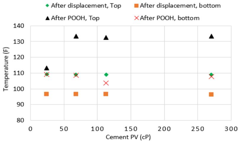
Figure 17: simulated slurry temperature influenced by cement's viscosity (PV). In all cases, YP is unchanged.
