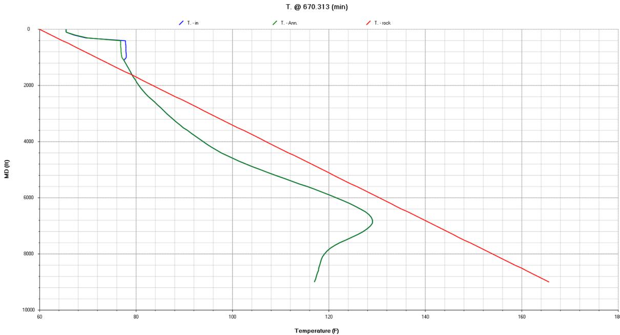
Figure 4: the fluid temperature at the end of POOH (pipe is at 1000 ft). Note the fluid below 8000 ft is noticeably recovered to a higher temperature if we compare it with the previous Figure.
