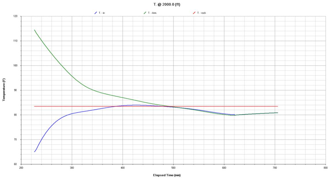
Figure 5: temperature history at 2000'. The T-in and T-ann merges to the same temperature at about 620 minutes, when the pipe end is pulled to the depth of 2000'.
