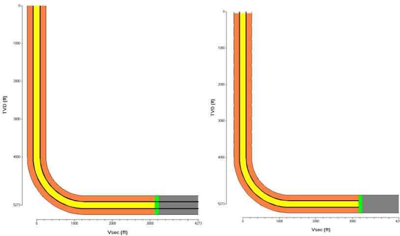
Figure 20: 2D schematics in a horizontal well showing the fluids after displacement (left) and after POOH (right) in the balanced plug.
