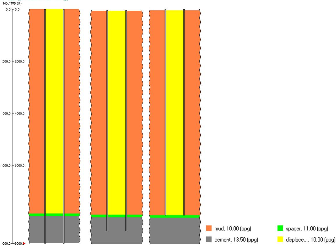
Figure 8: wellbore schematics with fluids during POOH. Left: the beginning of POOH (pipe end is at 9000 ft); middle: POOH when the pipe is pulled to 8500 ft; right: end of pull (pipe end at 8000 ft). [adjust the graph to align the top and bottom of the three wellbore schematics, and make the heights equal.]
