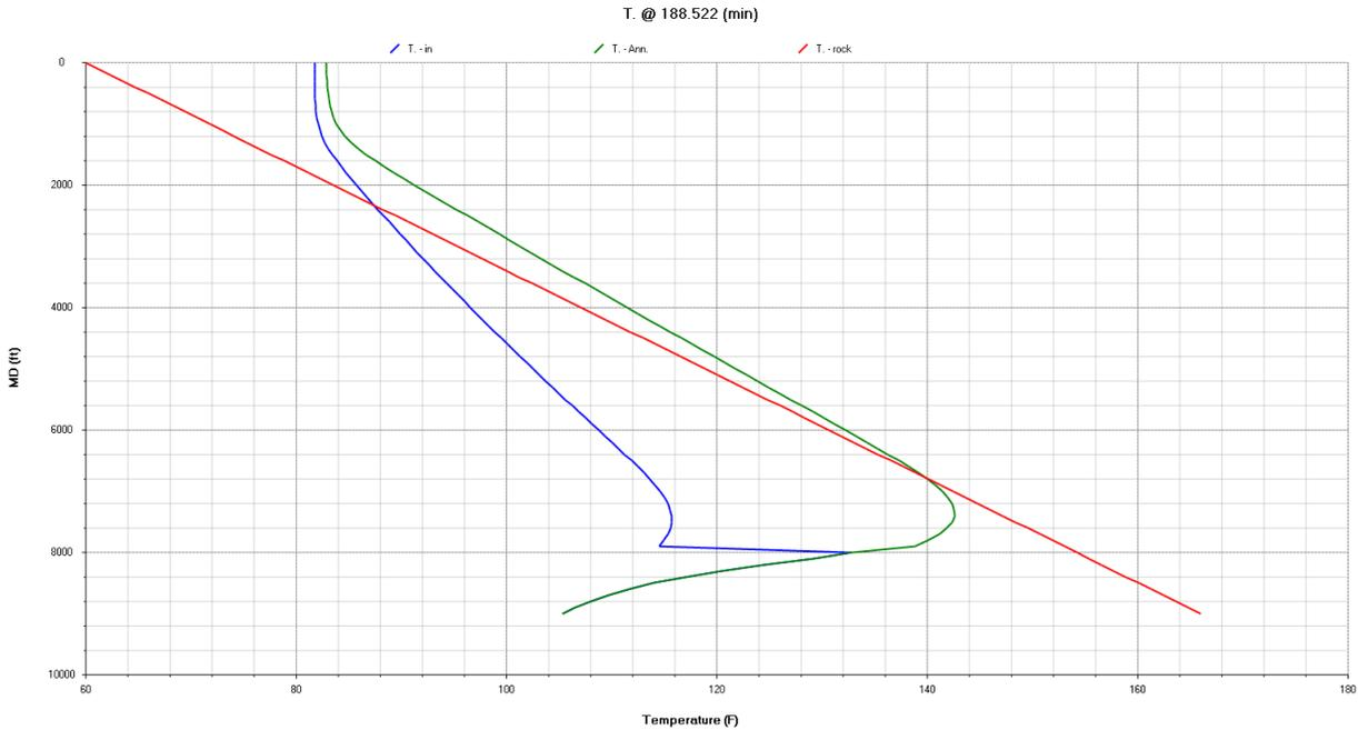
Figure 10: temperature profile after POOH (pipe end is at 8000').
