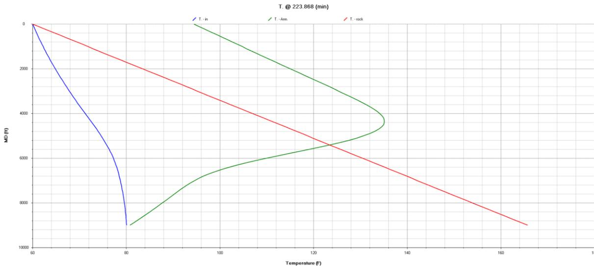
Figure 2: Temperature distribution after circulation. BHCT is approximately at 80 F.
