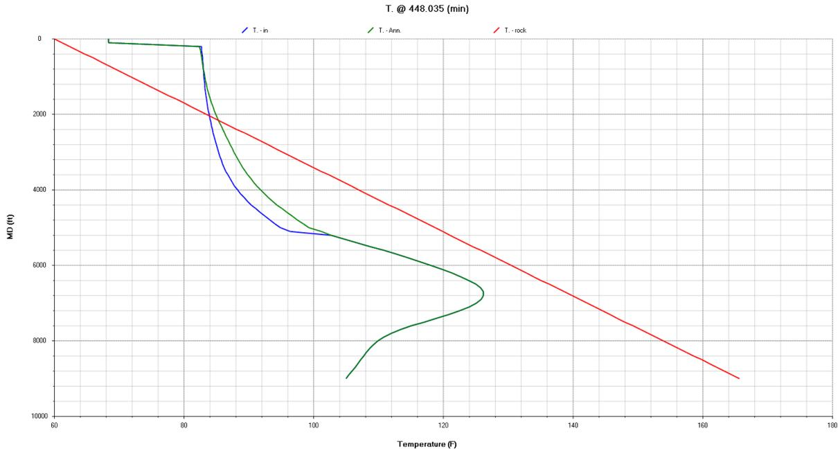
Figure 3: Temperature distribution when the pipe end is at 5000'. The fluid inside pipe at the pipe end runs out of the pipe and meets with the neighboring fluid dropped out of the annulus, and the mixed fluid is considered to reach a uniform temperature quickly (the time is ignored in the model). Therefore, for depths below the pipe bottom, T-in and T-annulus share the same line.
