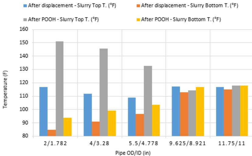
Figure 12: slurry temperature in a balanced plug job by various pipe sizes.
